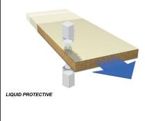
Pre Milling Unit 0.75 + 1.1kw 12000 RPM
