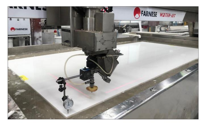
The machine includes an abrasive bucket for the abrasive inlet, with automatic feed and mixing disk, where the total volume is 100 litres. After the abrasive is mixed in the mixing chamber, the segments of the cuttings and the abrasive form a mud on the bottom of the cutting tank. This mud can be sucked out by a pneumatic diaphragm pump and the water can be reused to maintain the water level.
