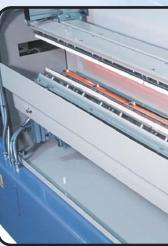
Four infrared heating banks control for thermic preparati glue coated substrate.
