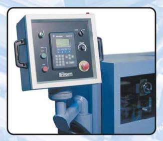
Space saving swivel mounted control console. User friendly console layout, with integrated operator interface.
