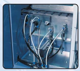
Full directional adjustment of spray nozzles for precise and even application of PVAC glue.
