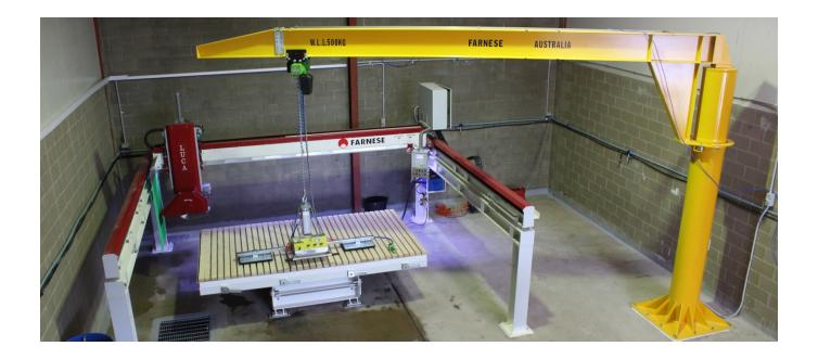
The JIB CRANE 360 is one of the most important elements in any mason's work shop.
