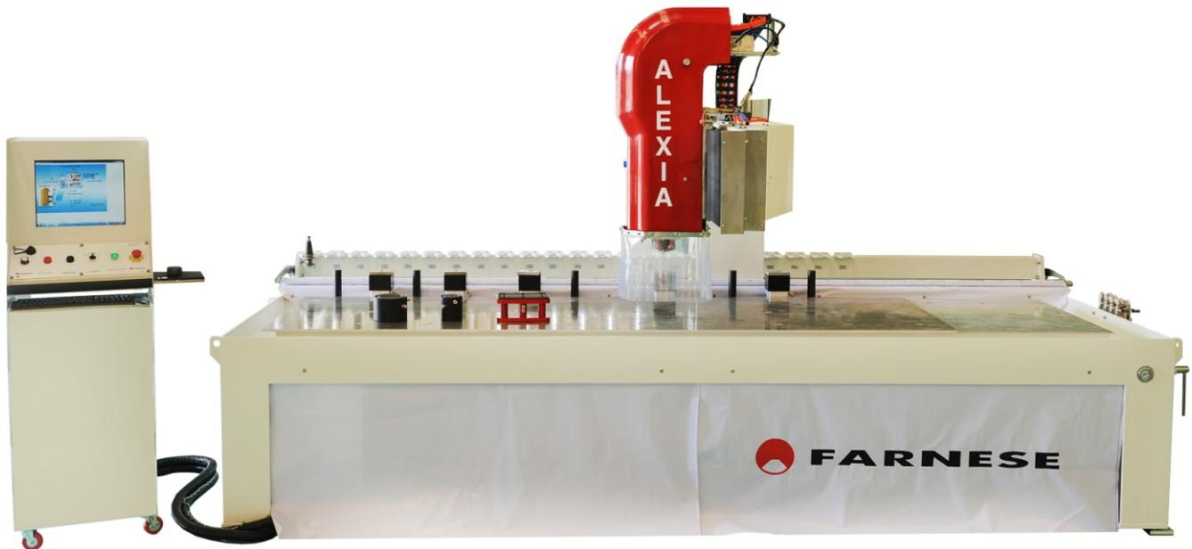
The ALEXIA automates the cutting, drilling and polishing of sink cutouts and is the ultimate answer to affordable stone processing without compromising on quality. The machine has automatic tool changing with 23 stations.
