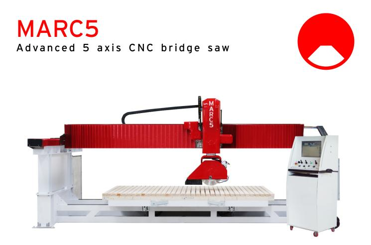
The MARC5 is the new breed of 5 axis bridge saws for the stone industry. It has a full CNC controller which coupled with the very easy to use front end program, makes this machine one of the most versatile saws available in the market. One of the great features of this machine is the fact that head/ blade can rotate around the full 360° and thus allowing the operator to make angled and circular cuts as well as tilting from 90° to 0° for drop in sink work.
